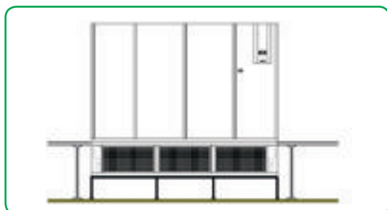
Unit with fan plenum installed under the raised floor.
